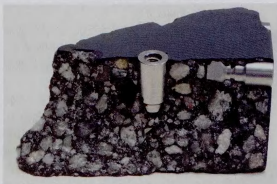
图1 带螺纹插件的结构 Fig.1 Structure of threaded metal insert
